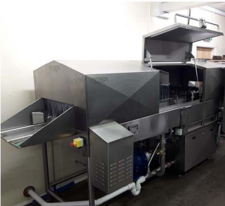
The machine was duly built and trials were carried out prior to despatch, in the presence of Sweet Moments, to determine if the wash quality was acceptable. Contaminated trays were transported from the Sweet Moments production facility, and washed to ensure the effectiveness of the machine. The trays, on exit from the system were clean and debris free.
